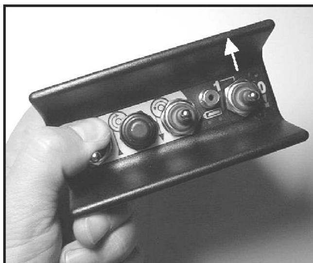
(pic 2.5-1 sog. “Resetting grip” of single-barrel transmitter)
