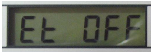
Figure 1: Example of deactivating the emptying function (Empty tank OFF).
