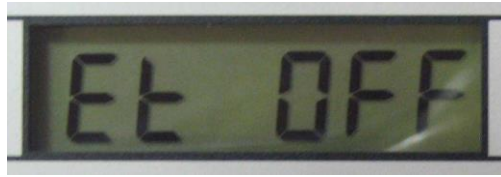
Figure 1 : Exemple de désactivation de la fonction de vidage (Empty tank OFF).
