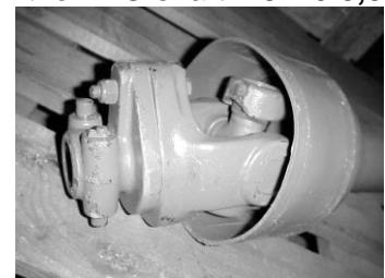
Shear bolt for the PTO shaft M8x40 8,8
