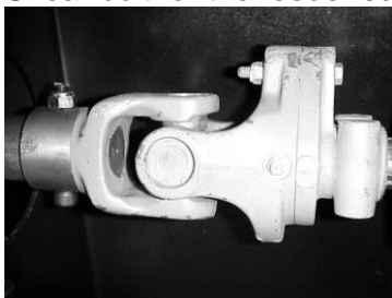
Shear bolt for the feeder screw M8x55 6,8
