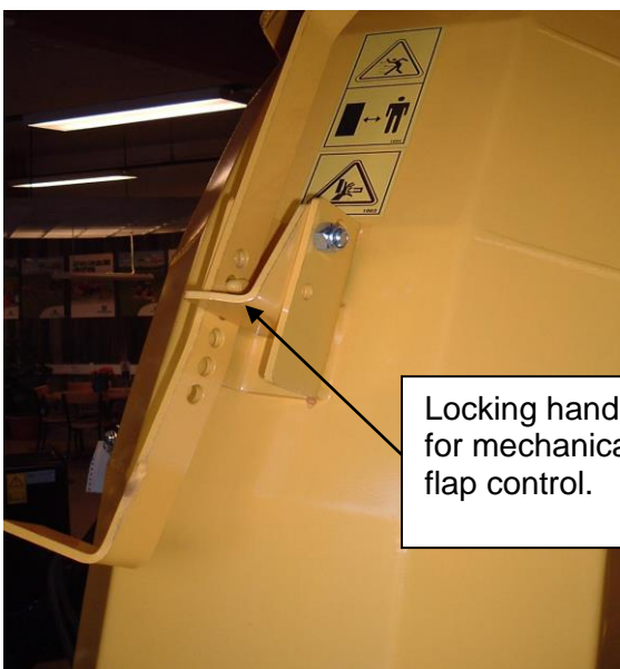
Mechanical flap control (Standard)
