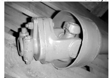
Shear bolt on PTO shaft M12x60 8,8
