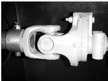
Shear bolt for the feeder screw M8x60 8,8
