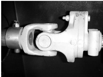
Shear bolt for the feeder screw M8x55 6,8
