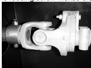
Shear bolt for the feeding screw M8x55 6.8 art. no. 970813
