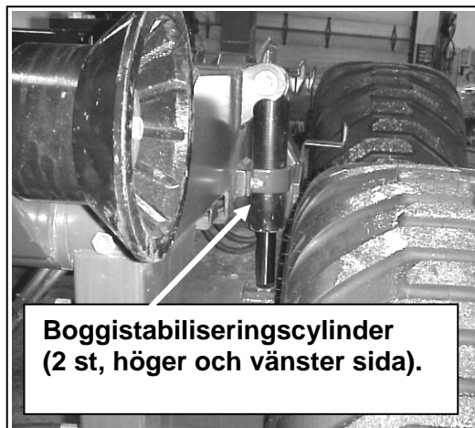
Fig.3a – Hydraulisk boggblockering
