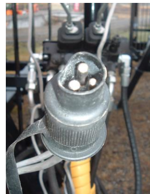
The crane's three-pole plug is connected to the outlet on the tractor (must be fused with 15 A). (Applies to cranes with lightweight package, EHC, PCL and radio control)
