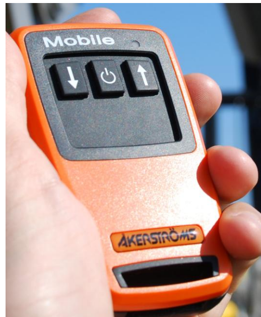
Portable unit radio control (for winch with buttons: on/off, in and out )
