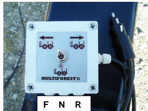
Hand unit (with automatic free wheel)
