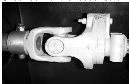
Shear bolt for the feeder screw M8x55 6,8
