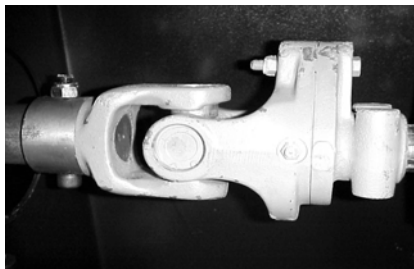
Shear bolt for the feeder screw M8x55 6,8
