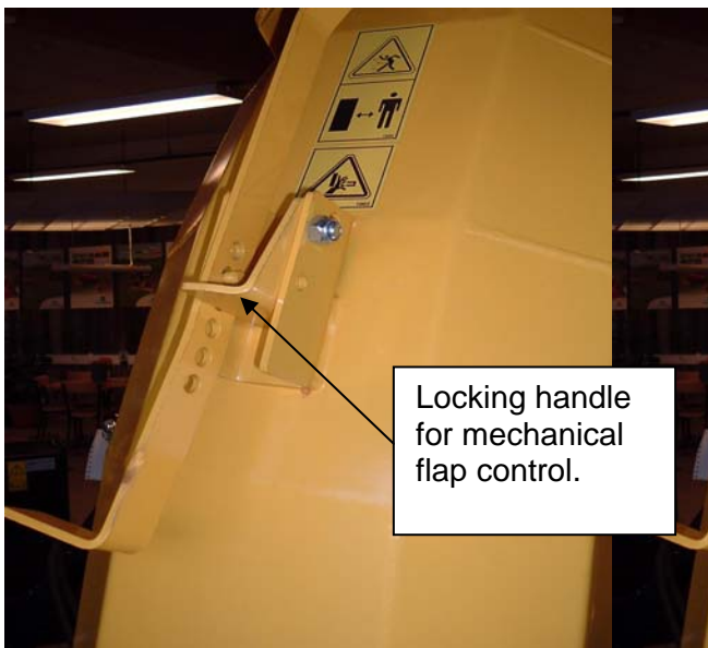
Mechanical flap control (Standard)
