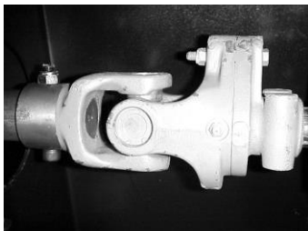
Shear bolt for the feeder screw M10x60 8,8
