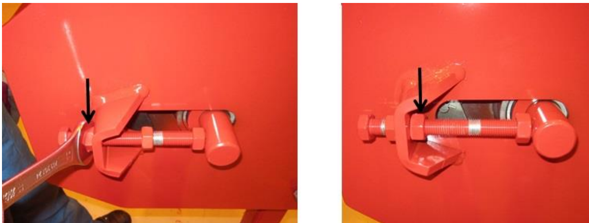
Figure 4 (Arrow left: tension, Arrow right: lock nut)
