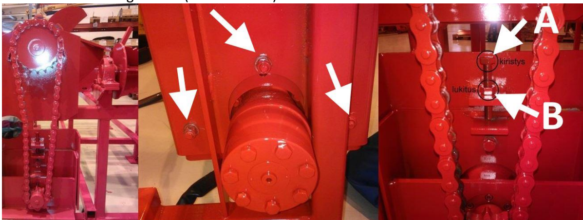
Figure 5 (tightening the motor chain)
