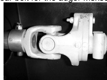
Shear bolt for the auger M8x55 6,8
