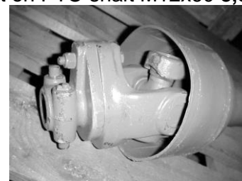
Shear bolt on PTO shaft M12x60 8,8
