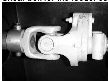
Shear bolt for the feeder screw M8x60 8,8
