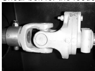
Shear bolt for the feeder screw M8x55 6,8
