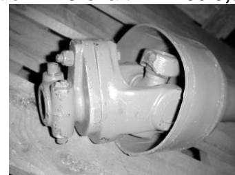
Shear bolt on PTO shaft M12x60 8,8
