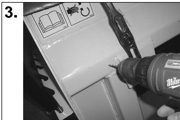
Drill a hole with 5 mm steel drill.
