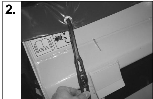
Place the plastic holder in the rubber strap and tension the strap towards a surface on the bucket suitable to fit each plastic holder. Mark were the hole should be drilled.
