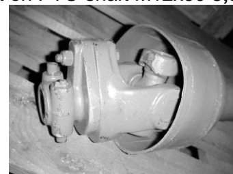
Shear bolt on PTO shaft M12x60 8,8
