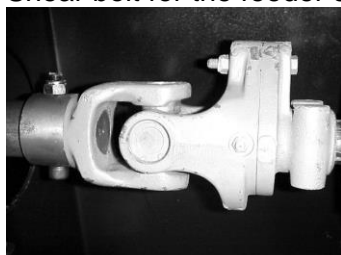
Shear bolt for the feeder screw M10x60 8,8
