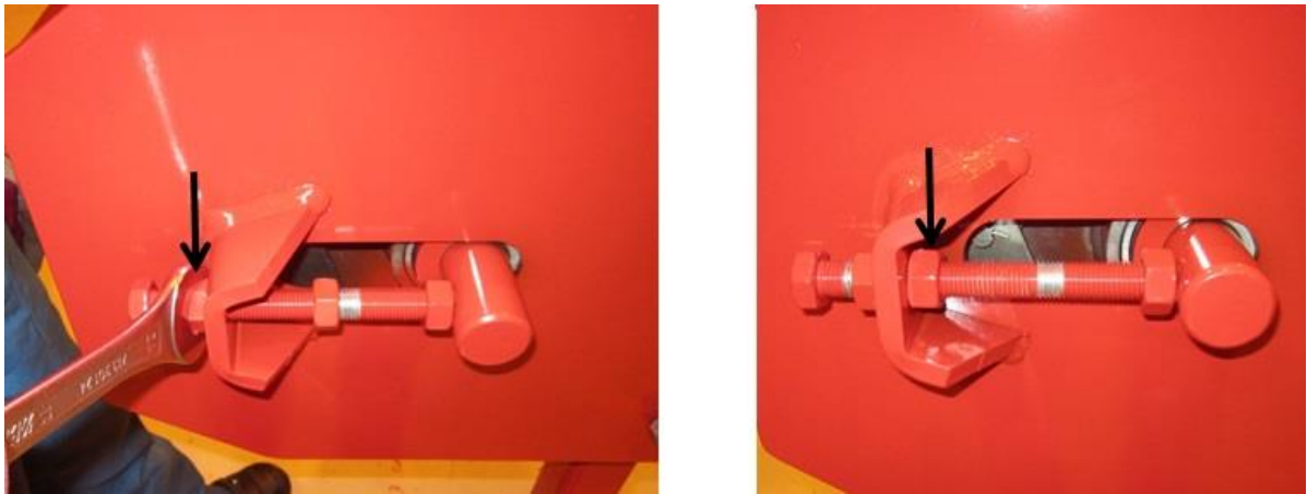
Figure 4 (Adjusting the tightness of the chain conveyor's chains)
