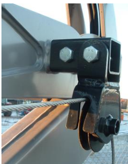
Deflection pulley 19-234 for mounting on crane arm.
