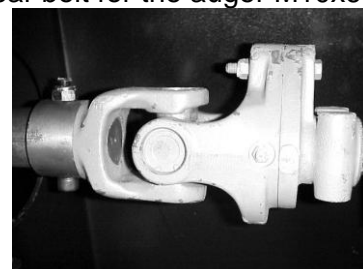
Shear bolt for the auger M10x60 8,8
