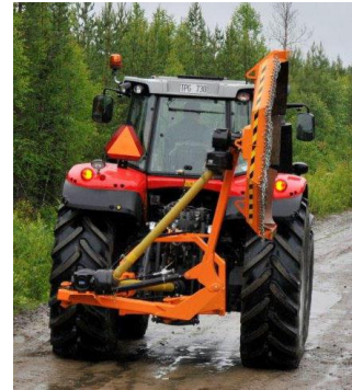
Draw in the side displacement arm so the transport width is minimised.
