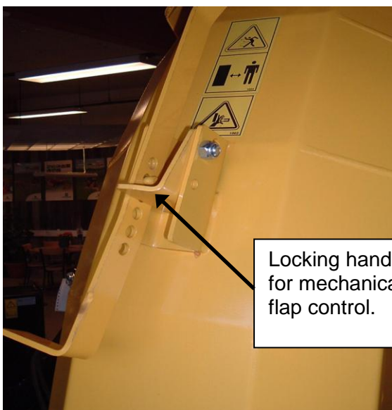
Mechanical flap control (Standard)
