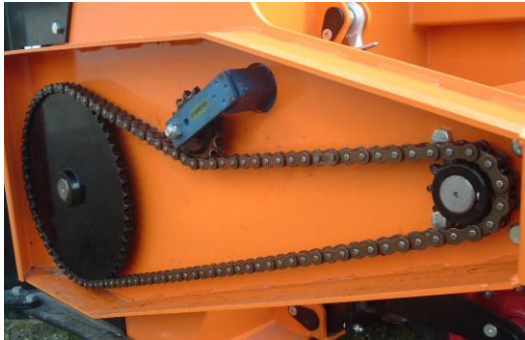
Auger chain drive with torsion tension device.
