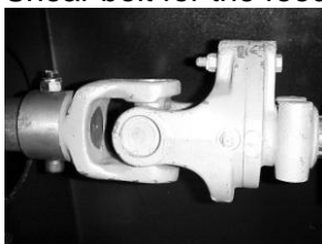
Shear bolt for the feeder screw M10x60 8,8
