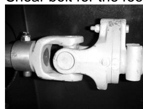
Shear bolt for the feeder screw M12x60 8,8
