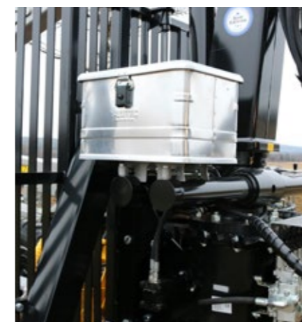
Toolbox Sturdy aluminum box, well protected placed behind the grille; 400x300x245 mm.
