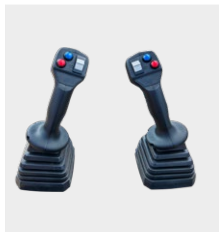
PCL Low Pressure Control Proportional control with 2 XY functions (PCL) including 4 electrical functions via slider and push button on the levers. The slide is used to control the telescope and gripper open/close proportionally.
