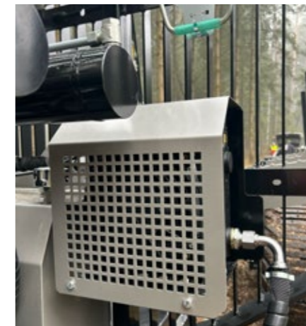
Oil cooler The electric oil cooler prevents thermal problems on long working days, not only in summer.
