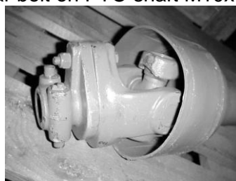
Shear bolt on PTO shaft M10x60 8,8
